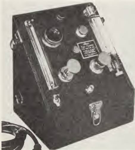
22-3. An instrument for determining the dewpoint temperature. (Illinois Testing Laboratories, Inc.)
